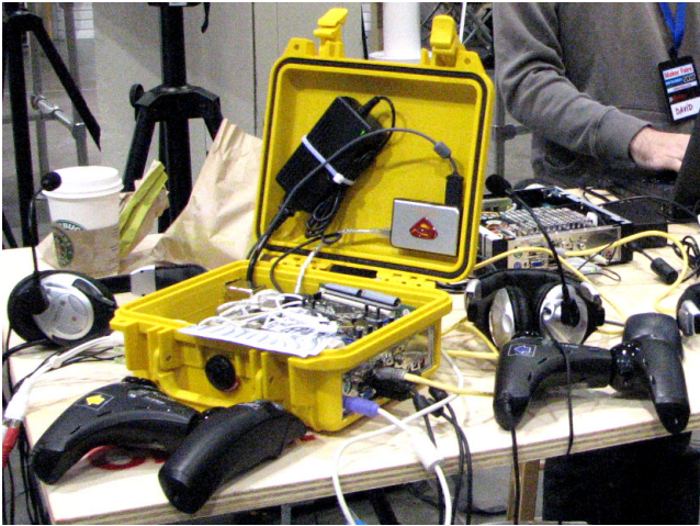
Figure 5: An Audiopint with the top open at the 2007 Maker Faire, showing its interior and surrounded by USB gamepads.
